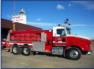
2641 2002 Kenworth Tender Seating Capacity: 2 Pump Capacity: N/A Tank Capacity: 3,000 Condition: Excellent Mileage: 12,132
