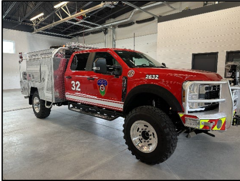
2632 2025 Ford F-550 Brush Seating Capacity: 4 Pump Capacity: 500 Tank Capacity: 400 Condition: Excellent Mileage: 3,432 Hours: 100
