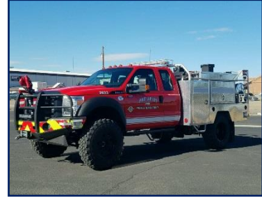
2633 2017 Ford F 550 Brush Seating Capacity: 2 Pump Capacity: 500 Tank Capacity: 400 Condition: Excellent Mileage: 4,392 Hours: 405
