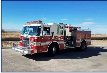
2606 1991 Pierce Dash Engine Seating Capacity: 6 Pump Capacity: 1,250 Tank Capacity: 750 Condition: Fair Mileage: 52,820 Hours: 4,308
