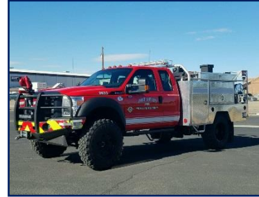
2633 2017 Ford F 550 Brush Seating Capacity: 2 Pump Capacity: 500 Tank Capacity: 400 Condition: Excellent Mileage: 6,535 Hours: 621
