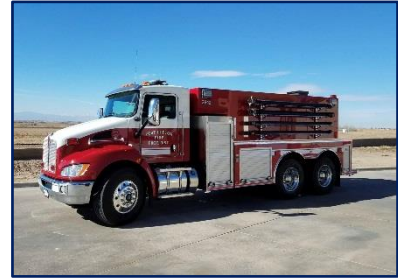
2642 2017 Kenworth Tender Seating Capacity: 2 Pump Capacity: 500 Tank Capacity: 3,000 Condition: Excellent Mileage: 4,970 Hours: 511
