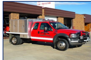
2631 2005 Ford F-450 Brush Seating Capacity: 4 Pump Capacity: 500 Tank Capacity: 400 Condition: Good Mileage: 10,191 Hours: 1,111
