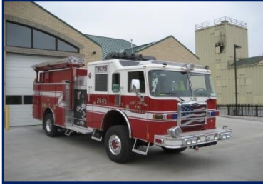
2605 2007 Pierce Dash 4 X 4 Engine Seating Capacity: 6 Pump Capacity: 1,250 Tank Capacity: 750 Condition: Excellent Mileage: 25,747 Hours: 1,933
